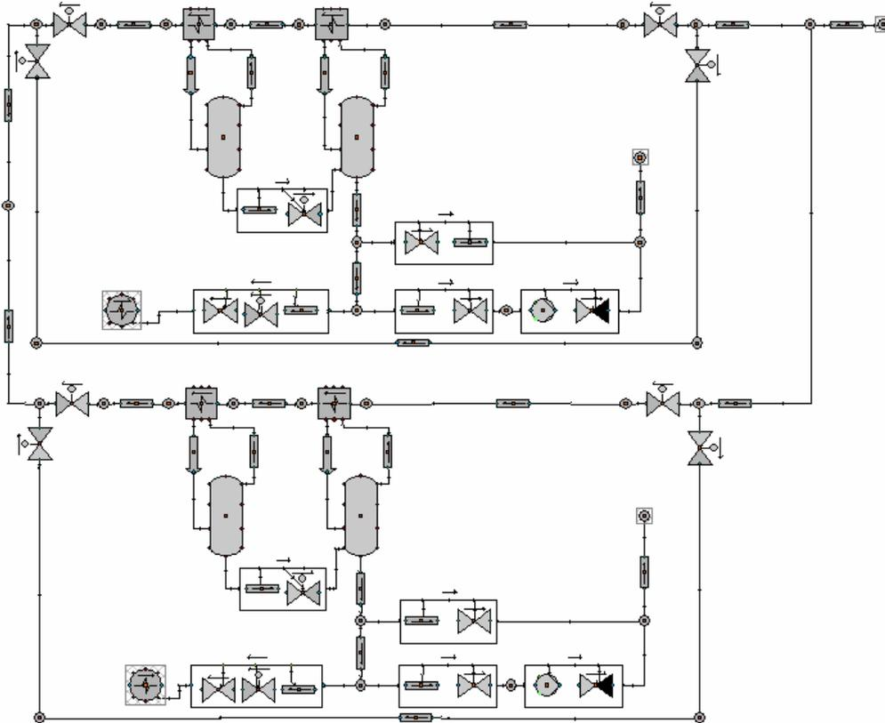
Figure 1. Part of feed water system of F2 as modelled in APROS graphical user interface GRADES
