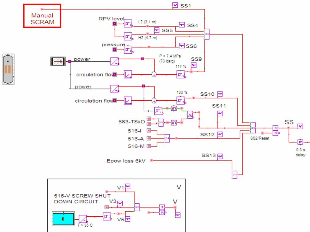
Figure 2. Part of reactor safety system of F2 as modelled in graphical user interface GRADES
