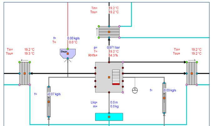
Containment node with connected heat structures and internal spray module.
