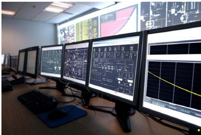
Figure 4: E&D simulator provides authentic environment for Apros model testing.
