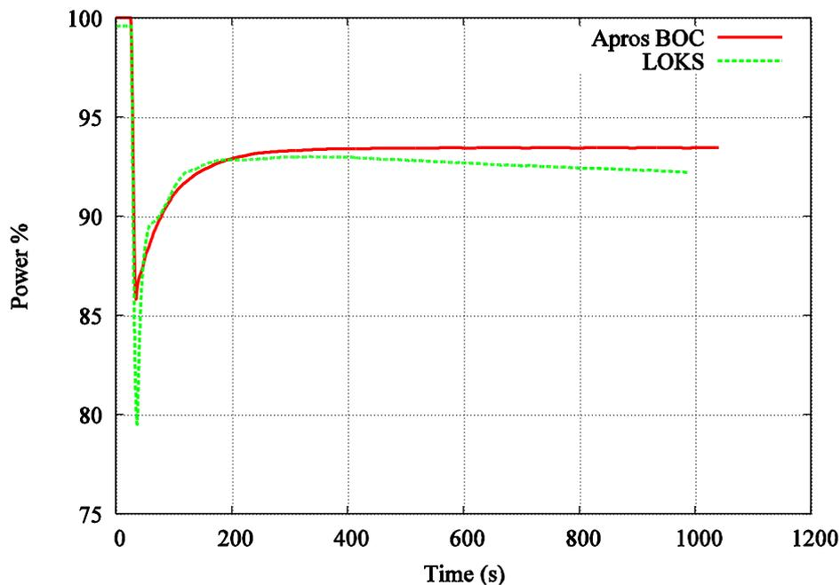
**Figure 5. APROS vs. old simulator (LOKS): Total power vs. time, Control rod drop, rod NCL207, group 6, BOC.**
