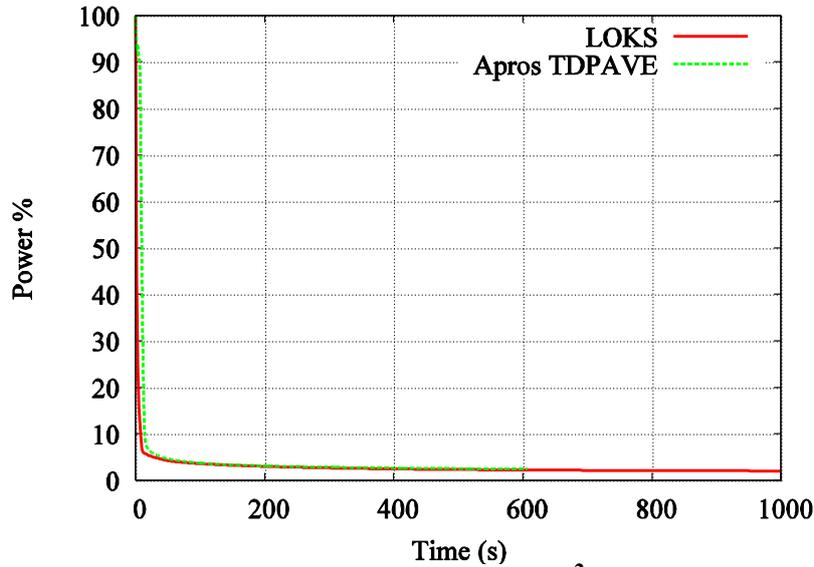
Figure 13. APROS vs. old simulator (LOKS): 200 cm<sup>2</sup> LOCA, Total power vs. time.
