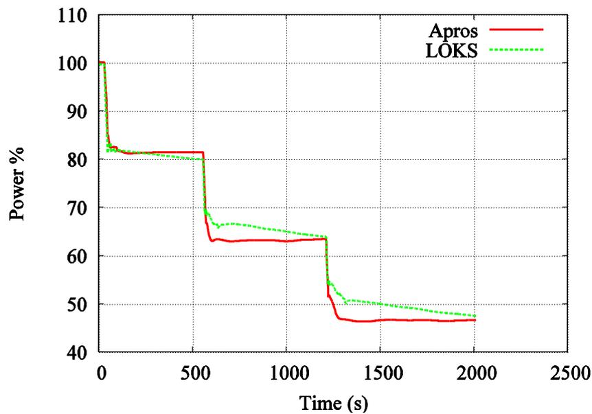
**Figure 10. APROS vs. old simulator (LOKS): Successive stopping of three main circulation pumps, Fission power vs. time.**
