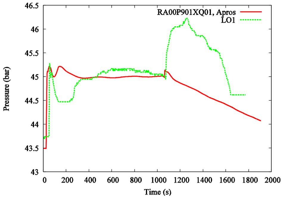
Figure 8. APROS vs. plant data (LO1): Stopping and starting of main circulation pump YD11D001, Steam pressure vs. time.
