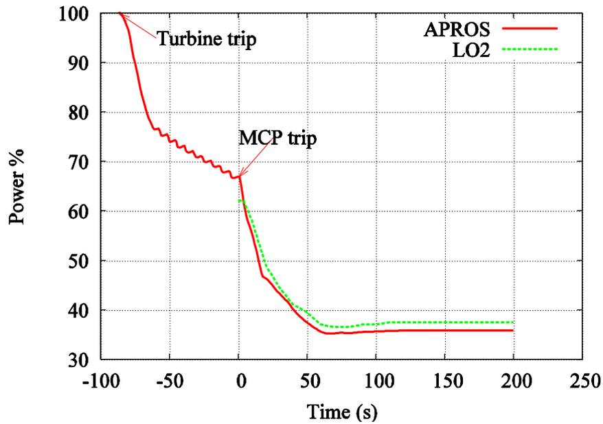
**Figure 9. APROS vs. plant data (OL2): Turbine trip and stopping of three main circulation pumps, Reactor power vs. time.**
