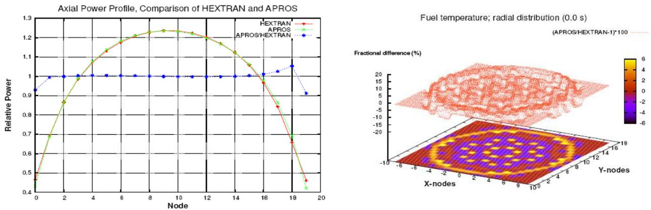
**Figure 1. APROS-HEXTRAN COMPARISON: Axial power profiles (left) and radial fuel temperature distribution (right) at steady state.**
