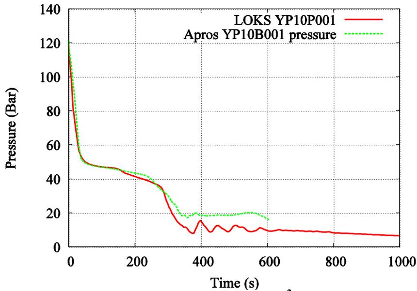
Figure 14. APROS vs. old simulator (LOKS): 200 cm<sup>2</sup> LOCA, Pressurizer pressure vs. time.
