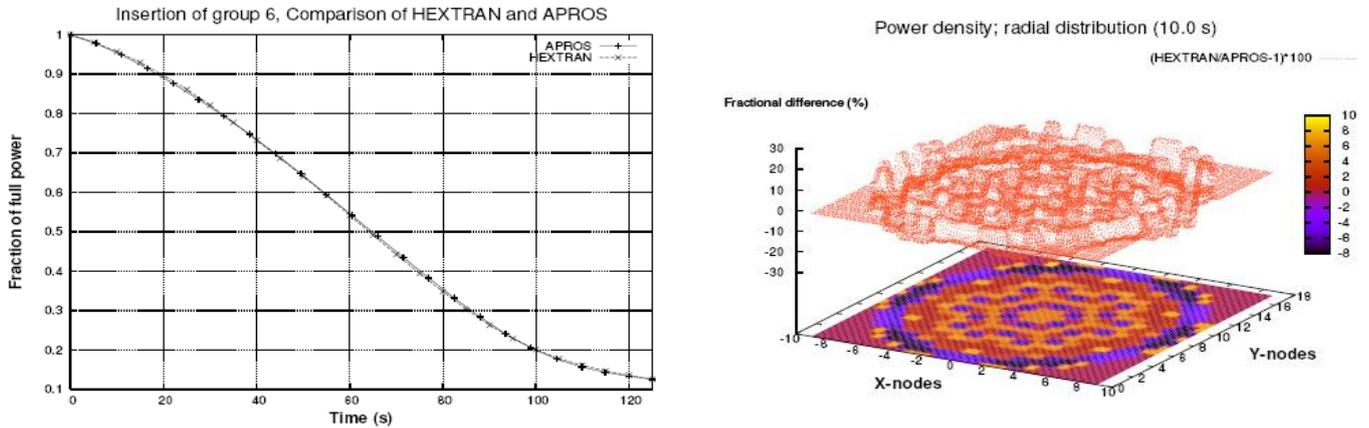
**Figure 2. APROS-HEXTRAN COMPARISON: Reactor power vs. time and fractional difference in radial power distribution at time 10 seconds during control rod group 6 insertion.**
