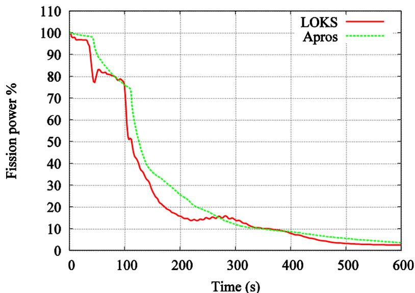
**Figure12. APROS vs. old simulator (LOKS): LOCA 20 cm<sup>2</sup> ATWS, Fission power vs. time.**
