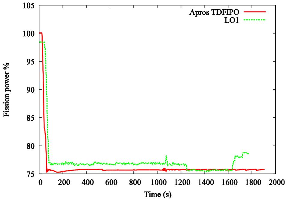
Figure7. APROS vs. plant data (LO1): Stopping and starting of main circulation pump YD11D001, Fission power vs. time.
