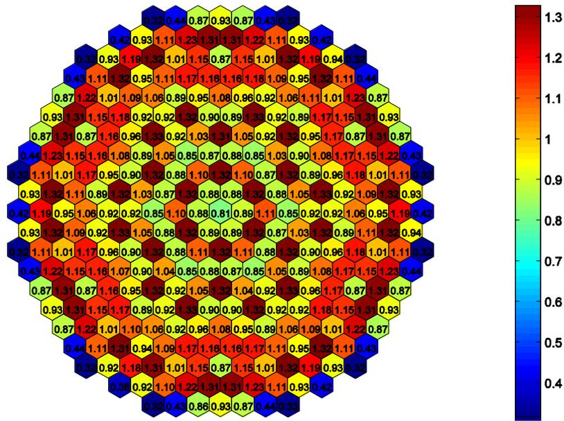
Figure 4. Radial power distribution at BOC.
