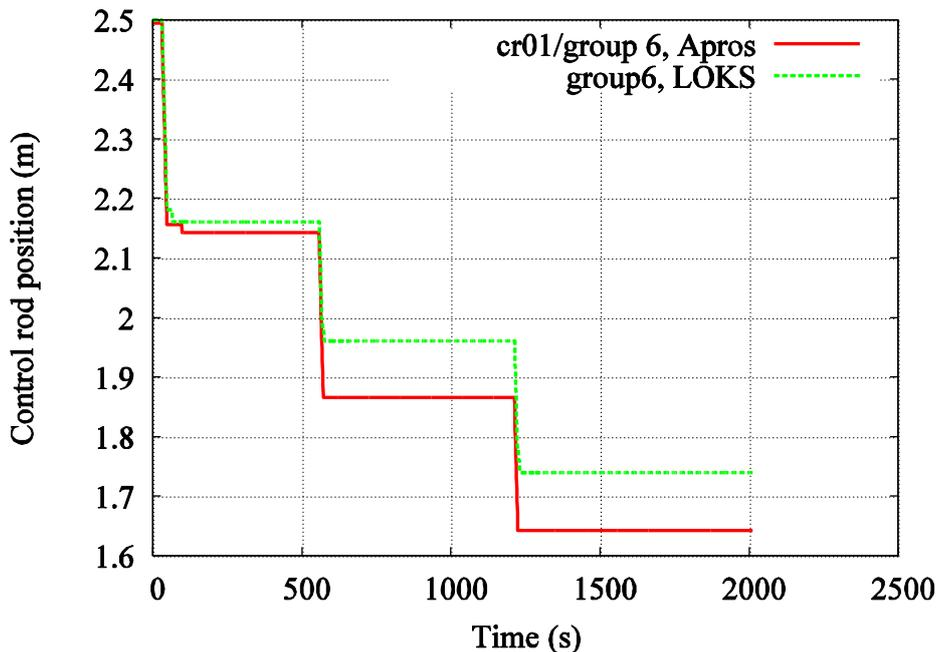
**Figure11. APROS vs. old simulator (LOKS): Successive stopping of three main circulation pumps, Control rod position vs. time.**
