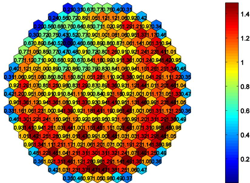
**Figure 6. Radial power distribution 15 seconds after control rod drop, rod 207, group 6, calculated with APROS**
