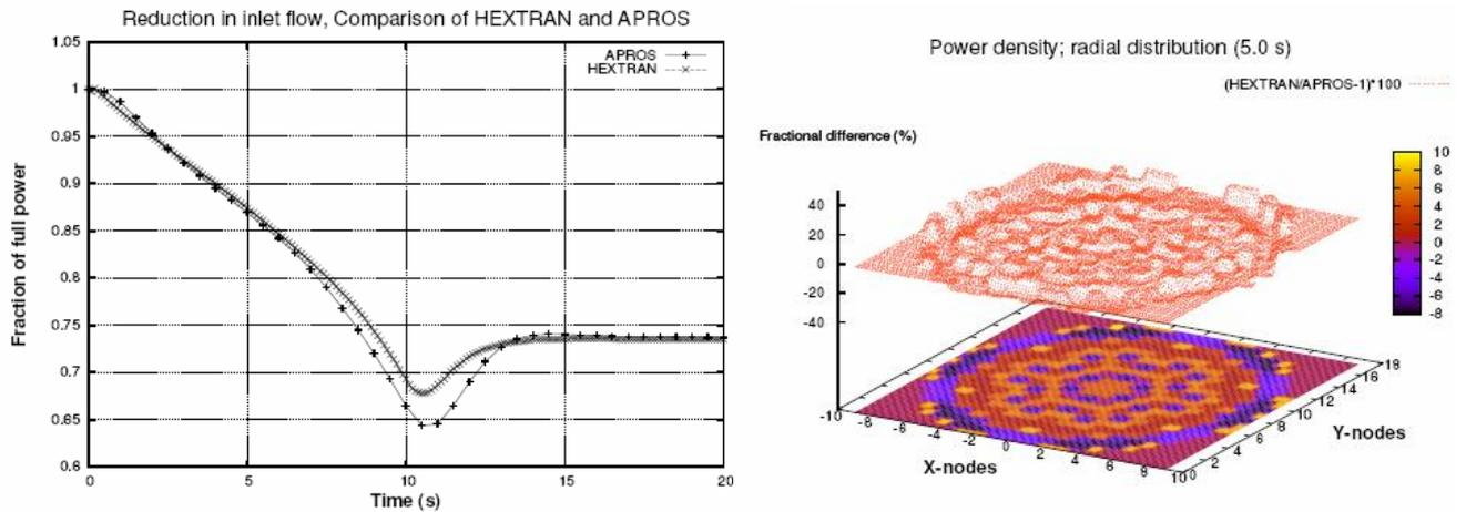
**Figure 3. APROS-HEXTRAN COMPARISON: Reactor power vs. time and fractional difference in radial power distribution at time 5 seconds during the reduction of coolant inlet flow from 100 % to 50 % in 10 seconds.**
