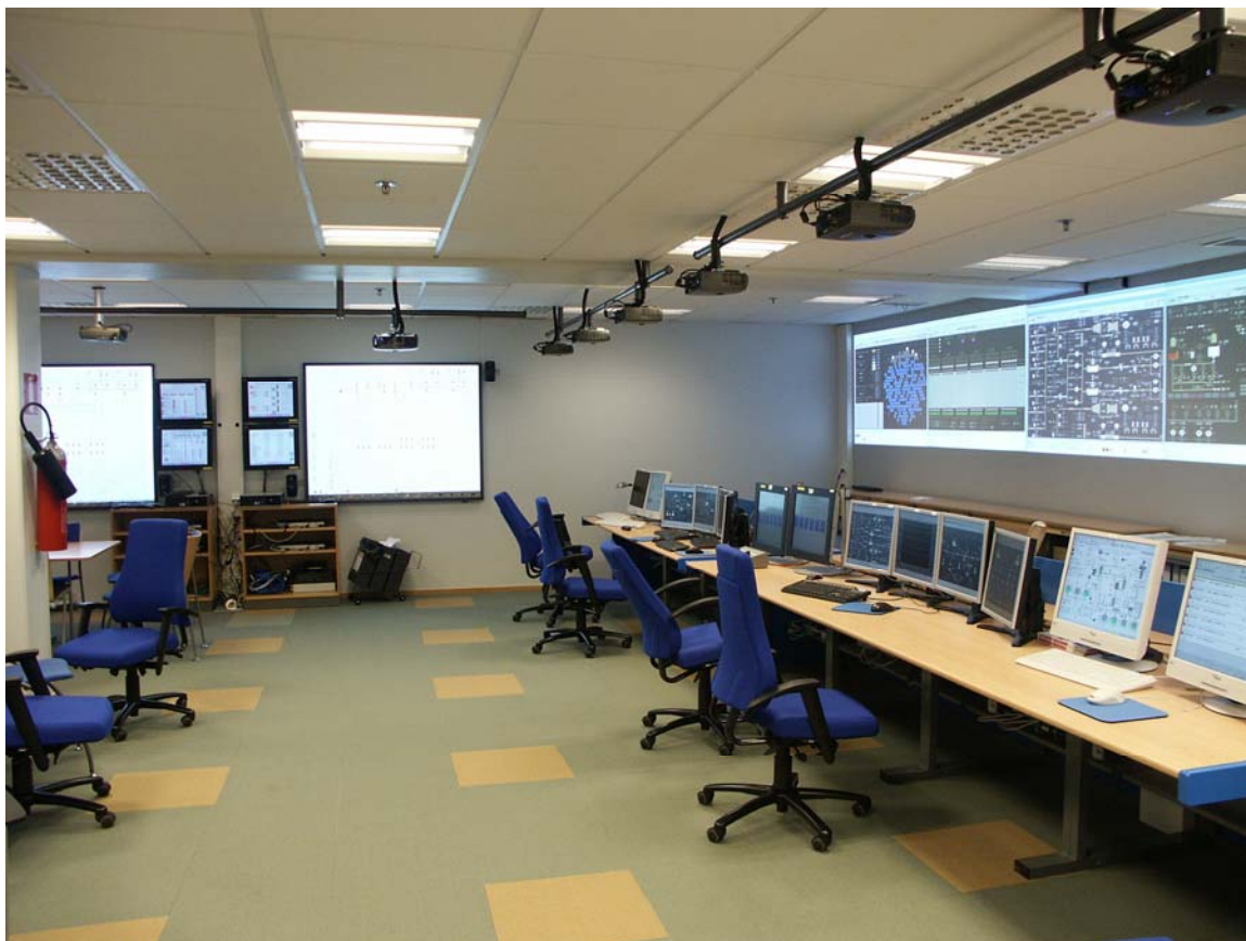
Picture 1. Development simulator in May 2009. Operator desk and large screen displays are on the right. In the back two large touch screens simulating hard wired panels of new reactor protection system and four QDS displays are presented.
